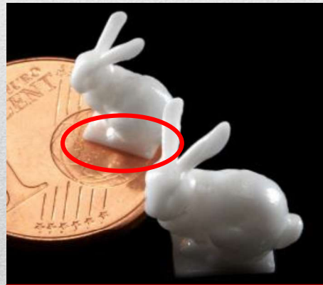
Lithoz's sample, there is a building plate on the bottom
